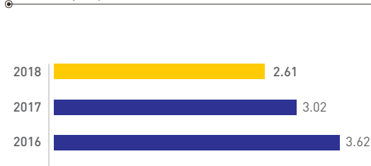
Dynamics of specific accidents rate at power grid facilities (number of technological failures (crashes) per 1,000 c.u. of equipment) of the Company in 2016–2018
